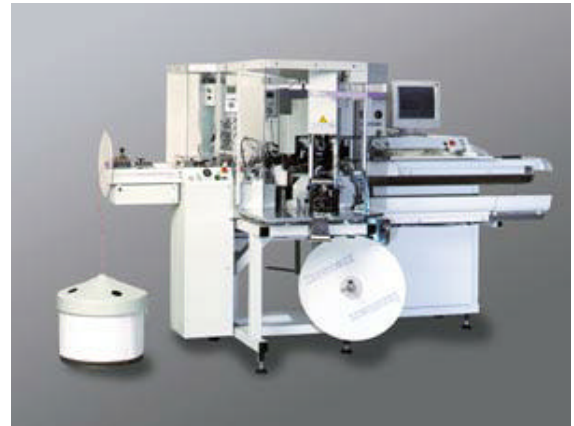
The komax gamma 333 PC with two mci 711 crimp modules and the mci 761 seal application module
